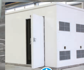
Unique composite GRP construction techniques allow INTERTEC to make lightweight shelters meeting stringent fire protection and safety requirements for offshore (or onshore) facilities - including EN 13 501-2 REI 120, UL1709 H90/H120 BS476, DIN 4102 F120. Fire resistant ceramic inner cores (below) can maintain internal temperatures below 60°C for up to 2 hours - even in hydrocarbon fires.
