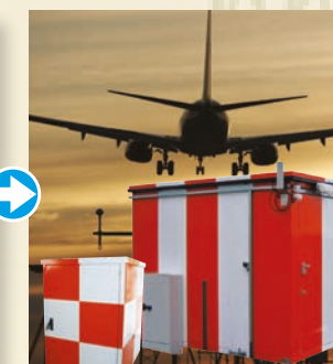
GRP cabinets using special construction principles to provide frangibility for equipment situated close to runways. 100% metal free construction additionally eliminates the danger of sparks on a collision and minimizes interference with radar/radio. GRP is also extremely light and fire retardant.
