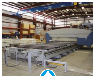
INTERTEC has the most sophisticated GRP manufacturing automation - including CNC machinery that can fabricate custom sizes in quantities as small as one, and in single-piece shapes to >12 m. This gives a major advantage in design flexibility - especially for larger shelters.
